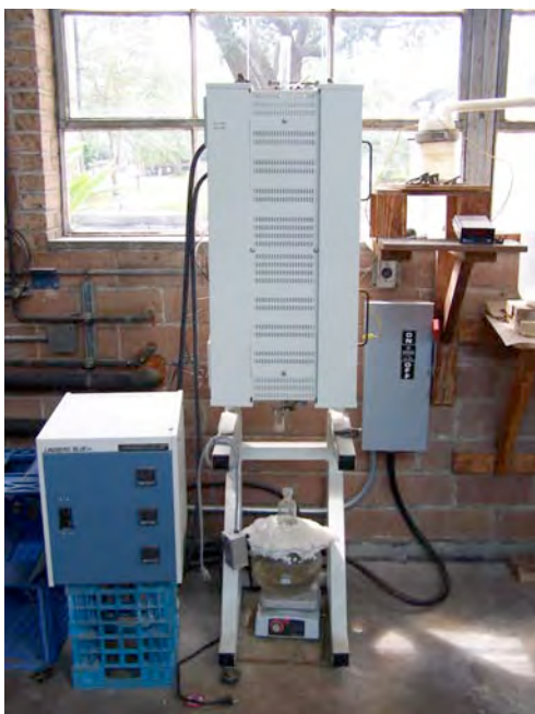
Figure 9. Lindbergh furnace with controller.
