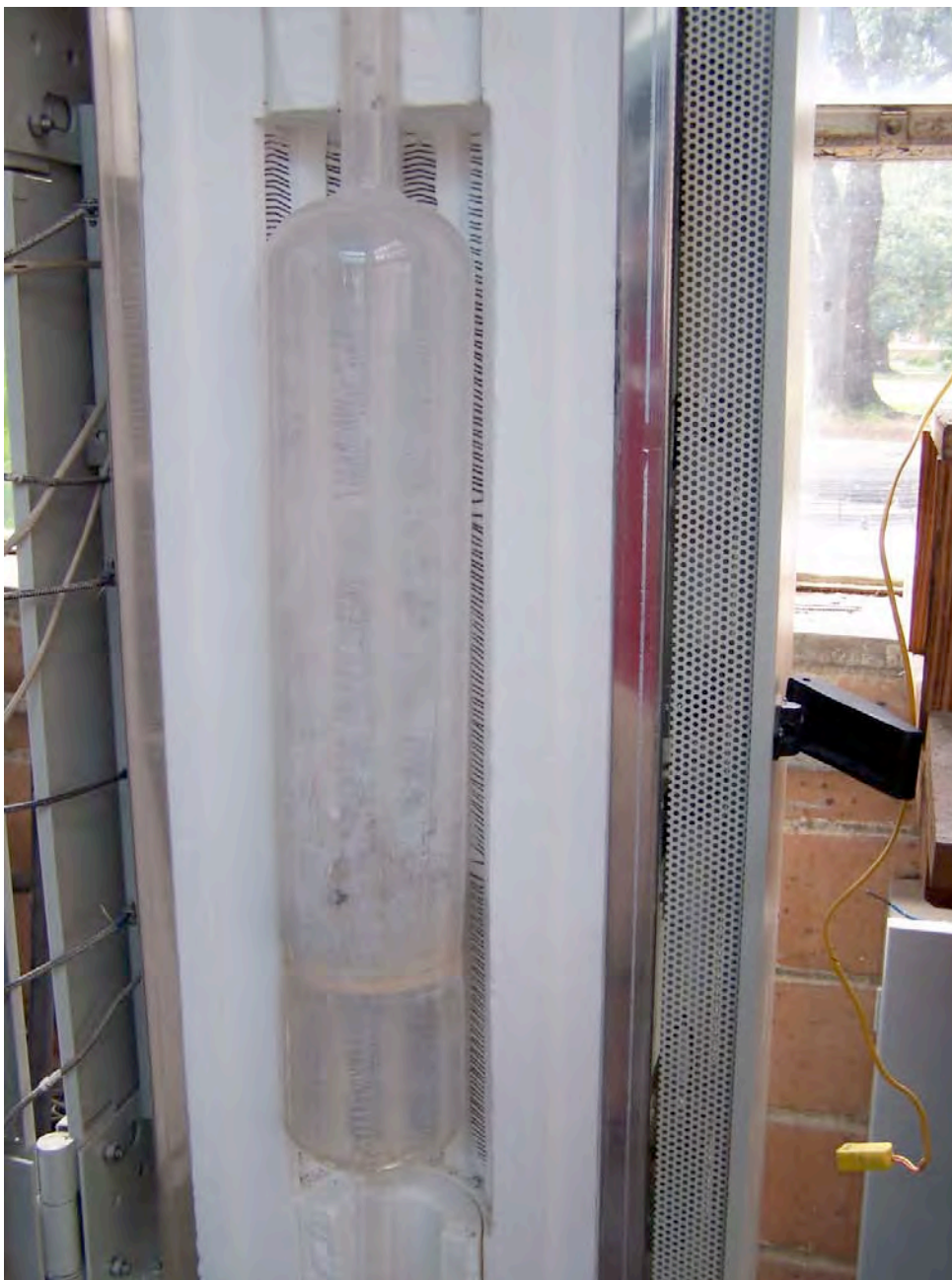
Figure 11. Close-up view of quartz fluidized bed reactor. Gas distributing fret appears in the lower portion of the reactor.
