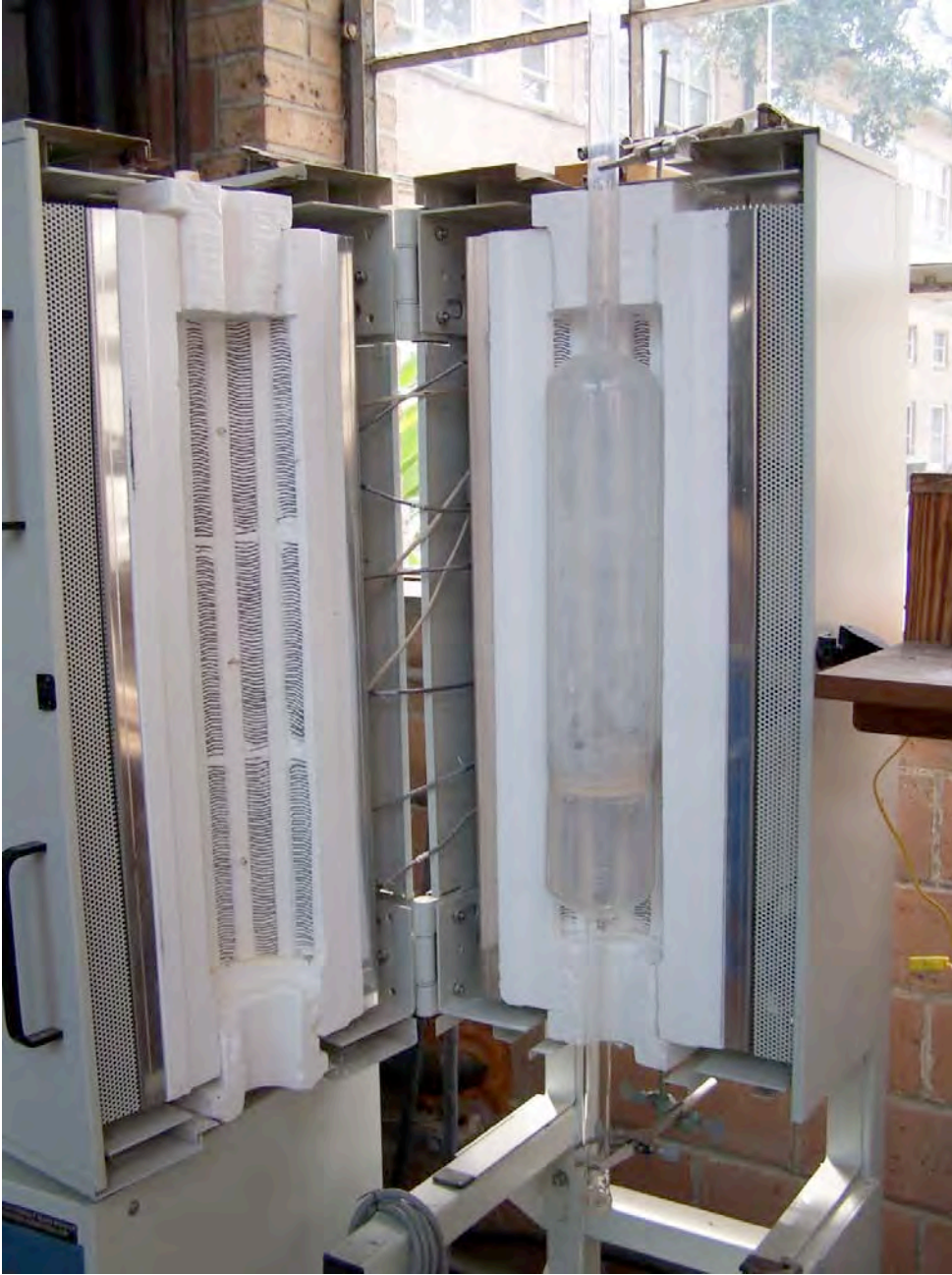
Figure 10. Open view of Lindbergh furnace showing quartz fluidized bed reactor.
